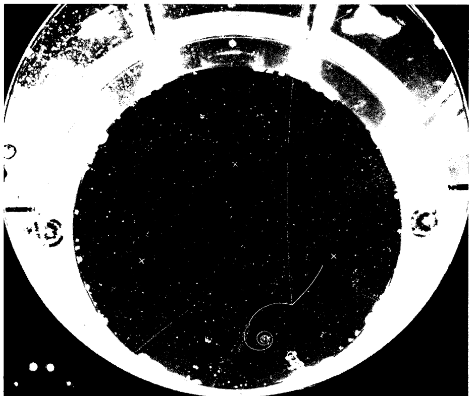
An example of a 'candidate' for a neutrino interaction with a 'free' proton. This interaction was observed for the first time in the recent series of neutrino experiments at CERN. The neutrino entering from the bottom of the photograph interacts with a proton (the nucleus of a hydrogen atom in the propane which filled the heavy liquid chamber) to give a proton (short track to the right) a muon (long upward track) and a positive pion which decayed eventually into a positron (the tight spiral).
